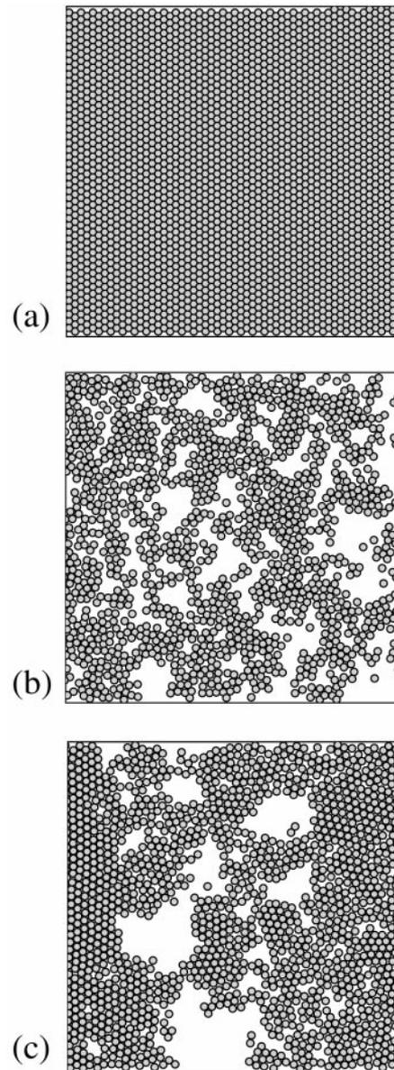
**Fig. 5a–c.** Snapshots from two-dimensional simulations that provide molecular level pictures of a initial two-dimensional configuration before irradiation with laser pulse, b homogeneous decomposition of irradiated material due to the phase explosion and c heterogeneous photomechanical disintegration. The laser irradiation is directed from the right side of the pictures
