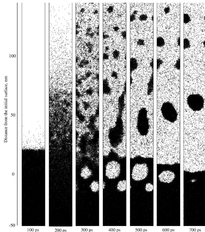
**Fig. 2.** A typical series of snapshots from the simulation in the ablation regime. The laser pulse duration is 150 ps, fluence is  $55 \text{ J/m}^2$ , and penetration depth is 50 nm. An animated sequence of the snapshots for this simulation can be found at <http://galilei.chem.psu.edu/~leo/Ablation.html>
