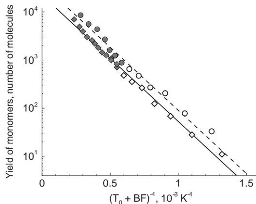
**Fig. 3.** Arrhenius plots of the yield of monomers from simulations with two initial temperatures. The *diamonds* and *circles* represent the data points for  $T_0 = 0$  K and  $T_0 = 500$  K, respectively. The *open* and *closed symbols* show the data points below and above the threshold for ablation. The *solid* and *dashed lines* represent fits of the data for  $T_0 = 0$  K and  $T_0 = 500$  K to the thermal desorption model (1) with the same activation energy of 0.52 eV
