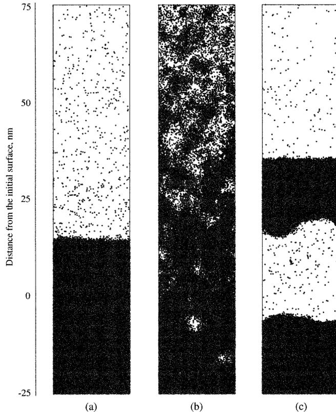
**Fig. 4a–c.** Snapshots from the simulations in the desorption (a) and ablation (b,c) regimes. The laser pulse durations are 150 ps (a,b) and 15 ps (c), fluences are  $34 \text{ J/m}^2$  (a),  $55 \text{ J/m}^2$  (b) and  $31 \text{ J/m}^2$  (c). The laser penetration depth is 50 nm in all simulations. The irradiation parameters correspond to the regime of thermal confinement in a and b and to the regime of stress confinement in c
